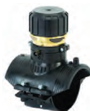
Stop-off Saddle (kit) Maximum passage 56.5 mm
